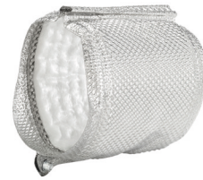
Embossed encapsulation of diesel particulate filter with flapped design, joined with screwing
